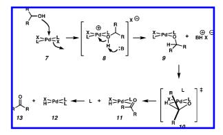
Figure 1. General mechanism of alcohol oxidation by palladium(II).
